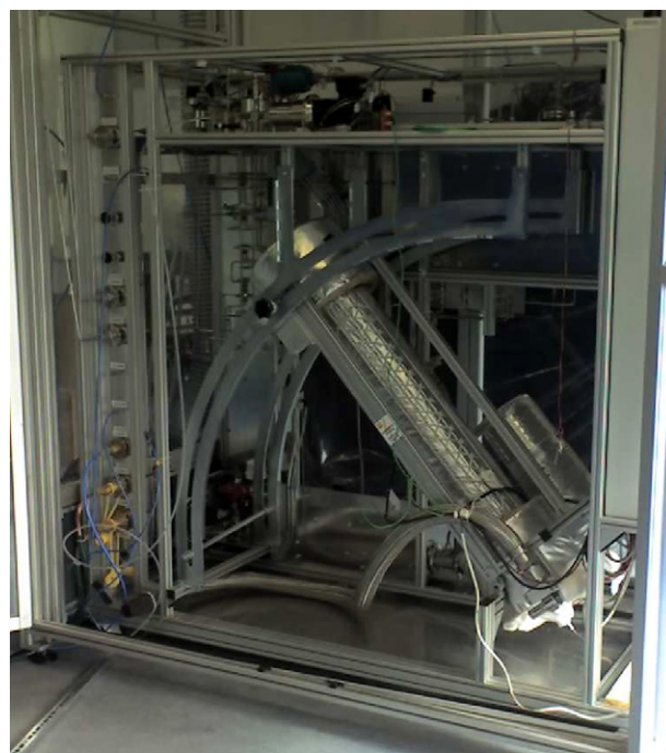
Fig. 4. POLF-HDS pilot-plant unit. The reactor position is at an angle of 45°.
